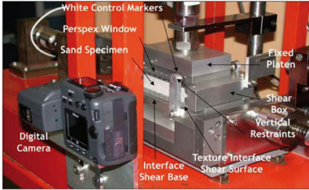
Figure 5. Apparatus for conducting constant normal stiffness shear box tests including digital imaging of the soil response.
