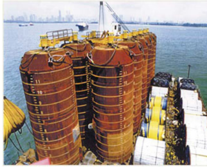
Figure 24. Laminaria suction anchors in transit.
